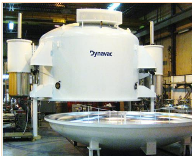
Figure 4 Dynavac mirror coating system for the Lowell Discovery Telescope
